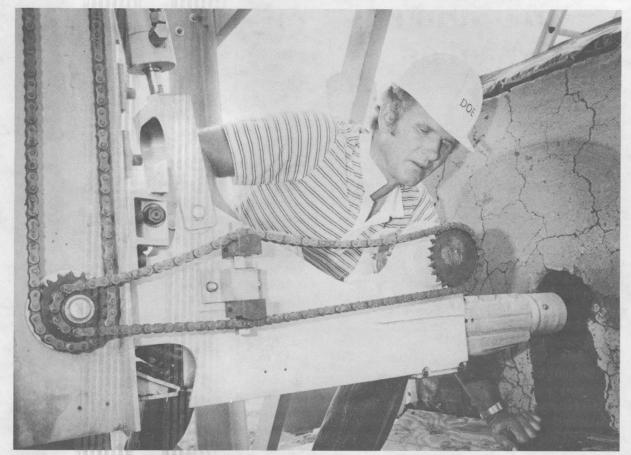
THIS DRILLING R&D relic being examined by Dave Shirey (5267) is the prototype cornering water-jet drill designed for use in coal mines. It died when funding for the Labs' fossil energy drilling program became a victim of budget cuts.
